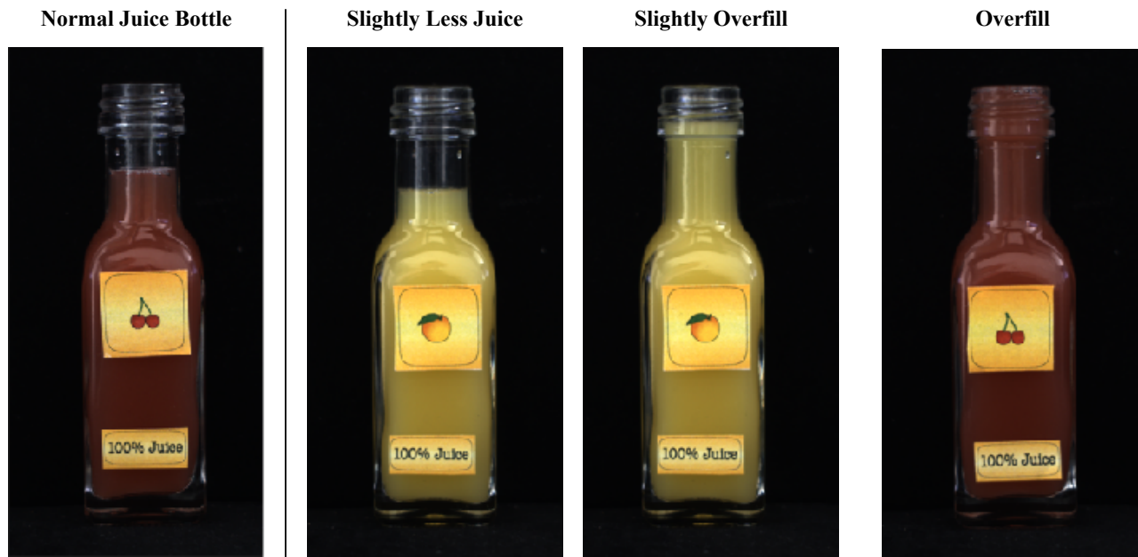
Figure 4: Failing cases: Juice Bottle in MVTec LOCO AD. AVLMs still encounter challenges in accurately determining the fill level of juice bottles. For example, bottles with slightly less juice and those with normal fill levels are nearly indistinguishable for AVLMs, even when utilizing the Guided CoT, such as, “is the juice filled to around half of the neck in the bottle?”. Note that these failing cases present significant challenges even for human observers.
