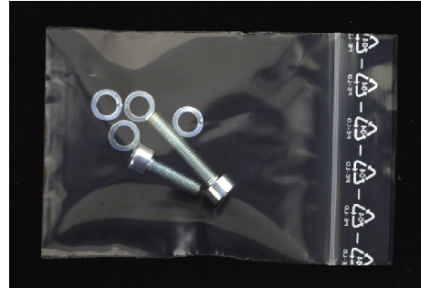
Figure 6: Failing cases, screw bag in MVTec LOCO AD. We observed that even with Guided CoT, “Describe the length of the shorter bolts, including the head, using the longer bolt as reference (only possible with 1/5, 2/5, 3/5, 4/5, and 1 of the longer bolt).”, the failing cases can still occur, same as “juice bottle”, these failing cases are also challenging for human observers.
